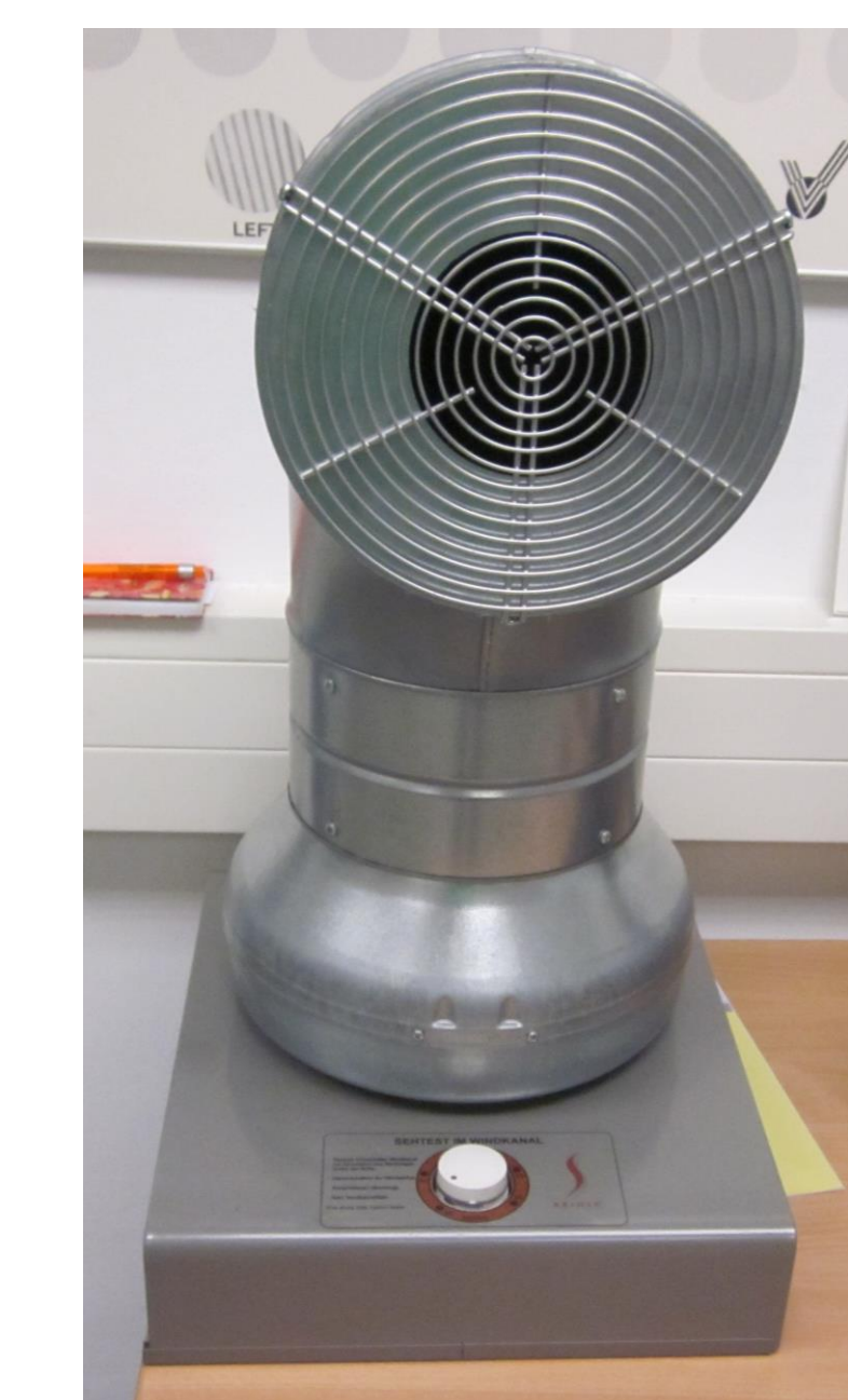
Fig. 3: Front view of the wind tunnel
