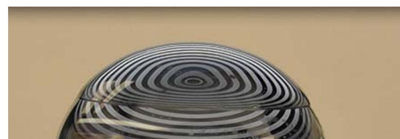
Figure 2: Ring reflection from wet lens surface
