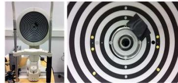
Figure 4: Keratograph 4 with test lens for the determination of magnification and region of interest
